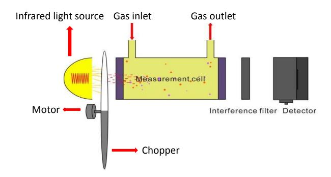
This spectroscopic method is based on the absorption of nondispersive IR radiation. The attenuation in the radiation which depends on the wavelength is a measure of the respective concentration of the gas.
